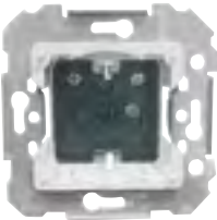
2P+E socket outlet (lateral earthing) with safety protection Screwed terminals 16 A 250 V~
