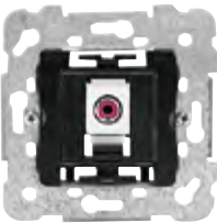
RCA mono socket outlet 18575 Rear screwless terminal. Cable: maximum 3 pairs of 0.3 mm² Pack of 1
