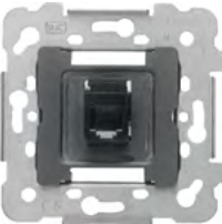
8-way female RJ45 connector Cat. 6 Tool-free connection by insulation piercing
