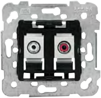
RCA stereo socket outlet 18576 Rear screwless terminal. Cable: maximum 3 pairs of 0.3 mm 2 Pack of 1
