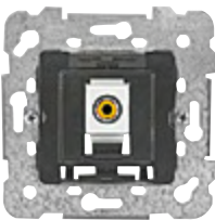
RCA video socket outlet 18577 Rear screwless terminal. Cable: maximum 3 pairs of 0.3 mm 2 Pack of 1
