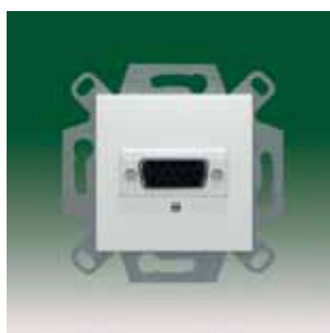
VGA connector 23578-VGA 15 pins D-SUB. Max. cable length 30 m. (depending on cable type) (screw terminals) Packing 1
