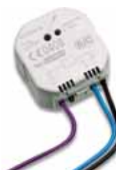
RF265625 Dimmer actuator plug-in 250 W incandescent and dichroic with electronic transformer. Not to be used with ferromagnetic transformers
