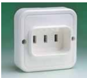
2P+E socket outlet 2225 White 25 A 250 V~ 85×85×35 mm Accepts any 2P+E plug 25 A 250 V~ S/UNE 20315 The terminals accept up to 10 mm 2 cables The most suitable box for this socket is ref. 2373-I Packing 5
